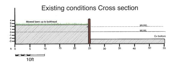
The existing conditions of the shoreline within the project area are mowed lawn up to a failing bulkhead with no connectivity to tidal water. Due to failing bulkhead sheets, tidal influence, and upland stormwater draining off the lawn, gaps and holes due to erosion have formed behind the bulkhead and continue to grow larger.
