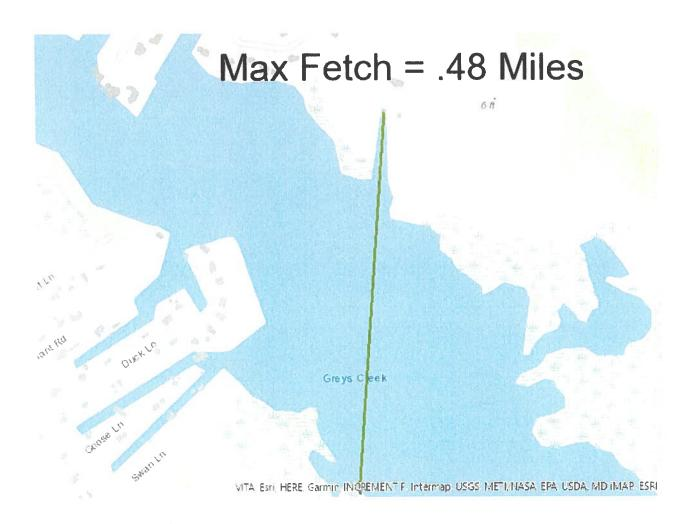
The project area has a low potential for wind driven waves given that it is at the end of a long narrow canal with a maximum depth of 3'. The only exposure is directly from the south with a maximum fetch of .48 miles. The living shoreline therefore does not need large structural components and can therefore focus on habitat creation and connectivity.
