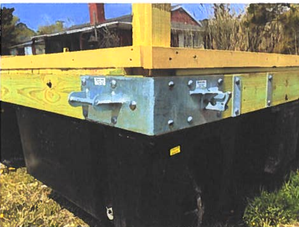
Raft units at storage facility showing wheeled floats, wooden edge walls, and the latch mechanism that connects rafts together.
